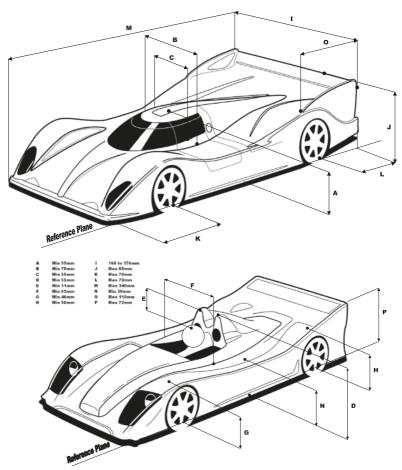
Once Homologated there must be no changes to the design, trim lines, detail lines or any feature of the body. All changes will require resubmission for approval and an additional revision letter added to the part number- Example 15001A - Original - 15001B for a 2ndRev. Etc
